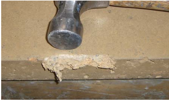
This “chip” was caused by repeatedly smacking the edge of the counter with a hammer. This is a good example for why we don't recommend you hammer on your countertop.
